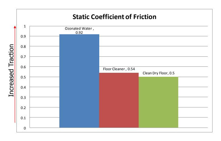
This study was conducted on an epoxy floor using the American Slip Meter (ASM 825). The higher the number, the more slip resistant the floor.
